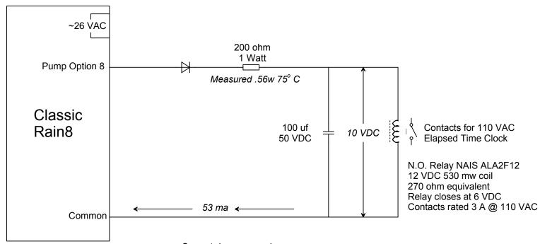
Current draw comparison: A Rainbird 24 VAC sprinkler solenoid measured 230 ma, 5 watts, 100 ohm equivalent
